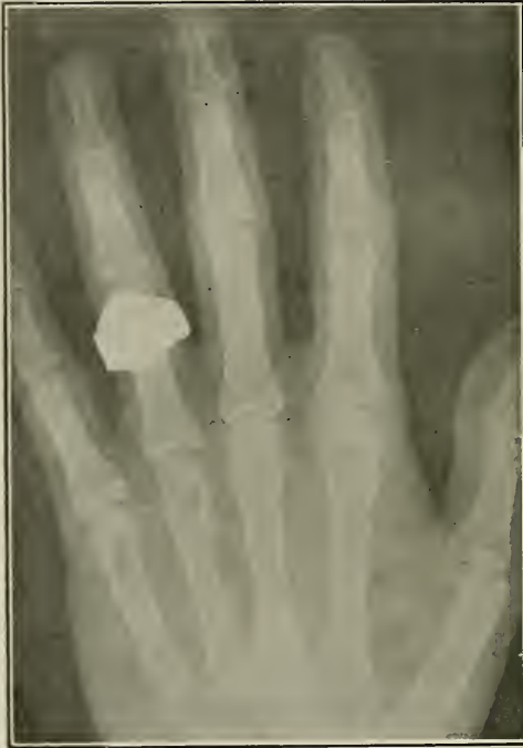
Fig. 108. Radiograph made on bromide paper. The conditions for making this radiograph were exactly the same as those given in Chapter IV for the negative of Fig. 71, except the time in the developer, which was about 100 seconds.
